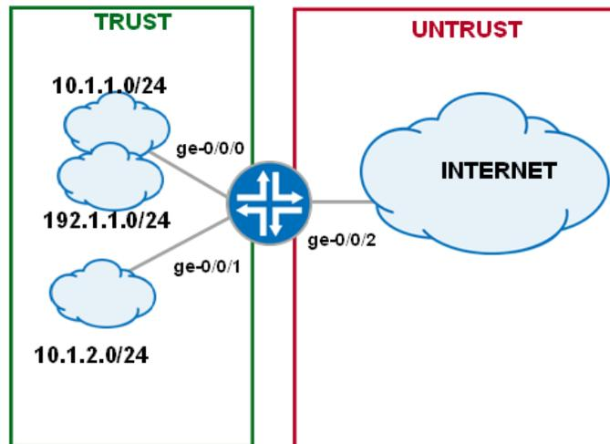
Fig1: source NAT using interface IP
